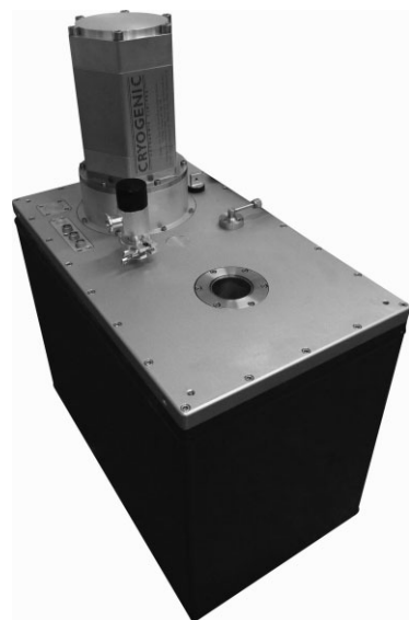
Figure 4. Cryogen-free desktop 7.05-T NMR magnet (300 MHz for ^1H isotope), with 0.2 ppm resolution and 54 mm room temperature bore [31].
