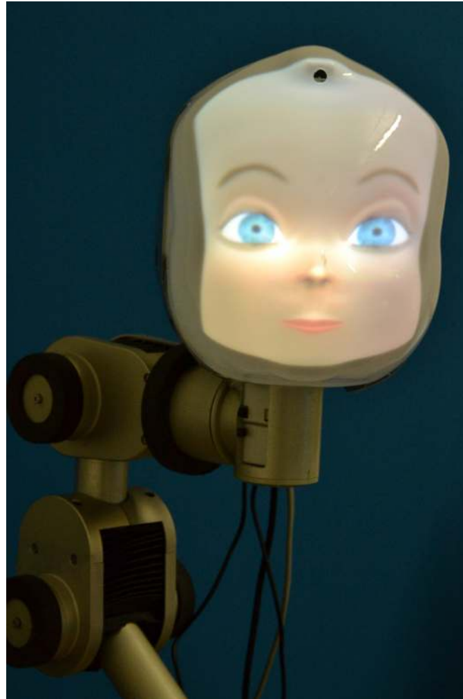
Fig 2. The LightHead robot. A semi-transparent mask mounted on a 6 DoF robotic arm, in which an animated character is projected.
