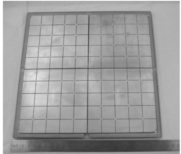
Figure 2. Electrode pattern of the bimorph mirror 260 mm \times 260 mm.
