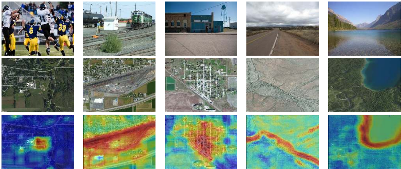
Figure 10: Examples of localization at finer spatial scales. (top) The ground-level query image. (middle) An aerial image centered at the ground location. (bottom) An overlay showing the distance between the ground-level image feature and the aerial image features at each location, computed using a sliding window approach (red: more likely, blue: less likely).
