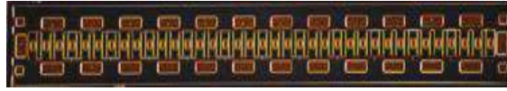
Figure 1. Photograph of a GaN high electron mobility transistor (HEMT) (CGHV1J070D) from Wolfspeed.
