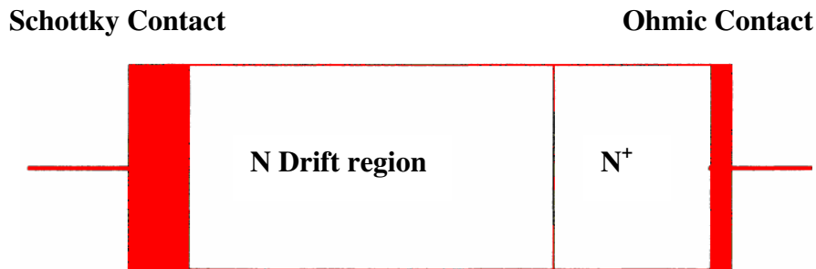
Fig. 2.1. Cross-section of a SBD.
