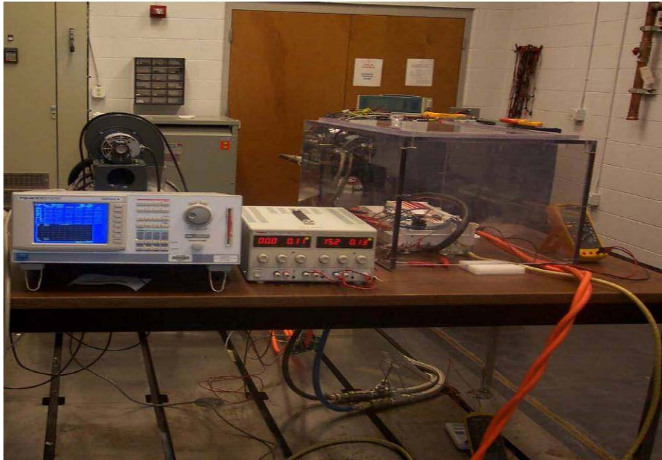
Fig. 3.20. Inverter dyne test setup.
