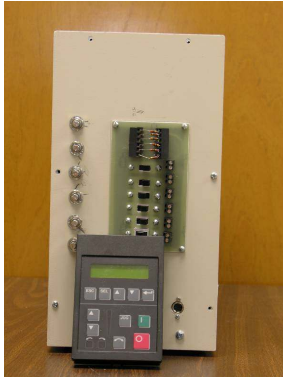
Fig. 4.20. Gate-drive control unit.
