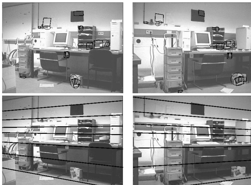
Figure 6: Example 2: final region correspondences (all matches correct) and epipolar geometry.
