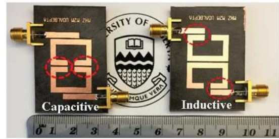
FIG. 6. Implemented capacitive and inductive coupled resonators to investigate and compare their dielectric sensing performance.
