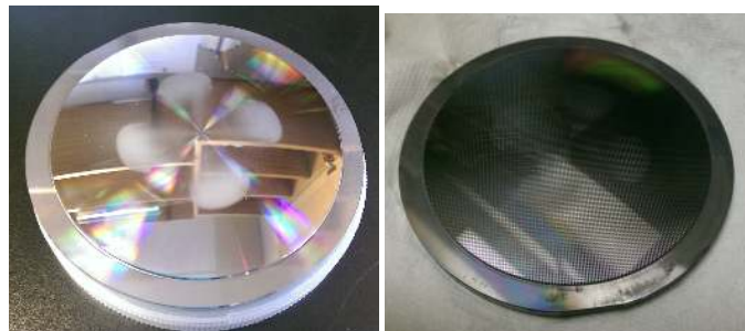
Fig. 7. Photos of the silicon lens prototype. Left panel: lens blank, which was produced by Nu-Tek Precision Optics using a CNC lathe. Right panel: lens after application of an AR surface layer manufactured using a 5-axis dicing saw. The outer diameter of the lens, including the outer ring used for mounting, is approximately 11 cm.
