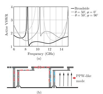
Fig. 15. (a) Common-mode resonances in the active VSWR of the array due to common-mode current excitation in the vertical feed lines; (b) schematic description of the common-mode current excitation.
