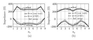
Fig. 7. Active input impedance for an array of (a)  $9\times\infty$  and (b)  $\infty\times9$  elements, at the frequency  $0.5f_0$  and as a function of the element index. The unit-cell geometry is defined in Tab. I.
