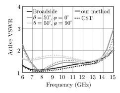
Fig. 9. Active VSWR of the array for broadside, scanning at  $50^\circ$  in E- and H-plane.
