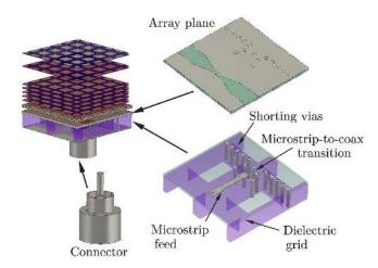
Fig. 17. A complete three-dimensional view of the unit cell array including the mini-SMP connector.
