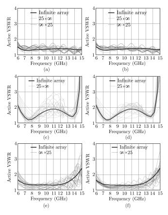
Fig. 13. Active VSWR of an array with  $25 \times \infty$  and  $\infty \times 25$  elements: (a), (c), (e) are relative to broadside, H-plane scan to  $50^{\circ}$  and E-plane scan to  $50^{\circ}$ , respectively, for uniform array illumination; (b), (d) and (f) refer to the same scanning conditions, but for a raised-cosine tapered illumination (6 dB edge taper).
