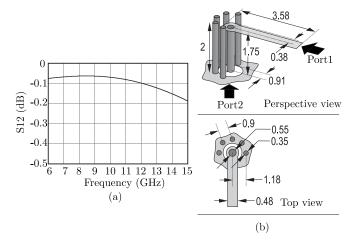
Fig. 14. (a) Transmission coefficient between ports 1 and 2 of the microstrip-to-coaxial transition; (b) geometrical parameters in mm.
