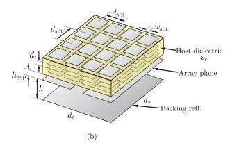
Fig. 2. (a) Connected array of slots in the presence of a backing reflector and (b) unit cell of the array loaded with ADL.
