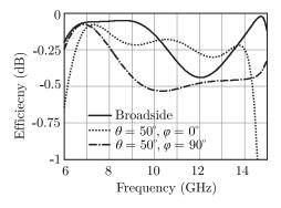
Fig. 19. The simulated efficiency of the array including ohmic and mismatch losses.
