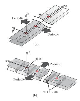
Fig. 6. (a) Finite  $\times$  infinite array of connected slots: (a) finiteness along x (H-plane) and (b) along y (E-plane).
