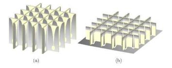
Fig. 1. Typical egg-crate configuration for wideband wide-scanning dual-polarized arrays: (a) tapered slot antenna array and (b) connected dipole array.
