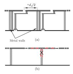
Fig. 16. (a) Introduction of the metallic walls to inhibit the propagation of the PPW modes; (b) current cancellation on the walls due to neighboring slots.
