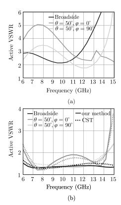
Fig. 12. (a) Deteriorating effect of the bonds on the active VSWR of Fig. 9; (b) re-optimized VSWR, accounting the effect of the bonds.
