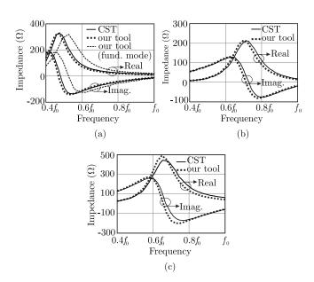
Fig. 5. Comparison of the input impedance of the connected array of slots loaded with ADL for (a) broadside, scanning to  $50^{\circ}$  in the (b) E- plane and in the (c) H-plane.
