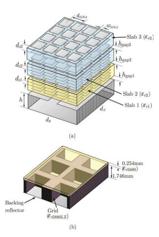
Fig. 8. (a) A unit cell of connected array radiating in the presence of multi-layer ADL stack; (b) exploded view of the dielectric stratification on the back side of the antenna.
