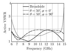
Fig. 18. Active VSWR of the array shown in Fig. 17.
