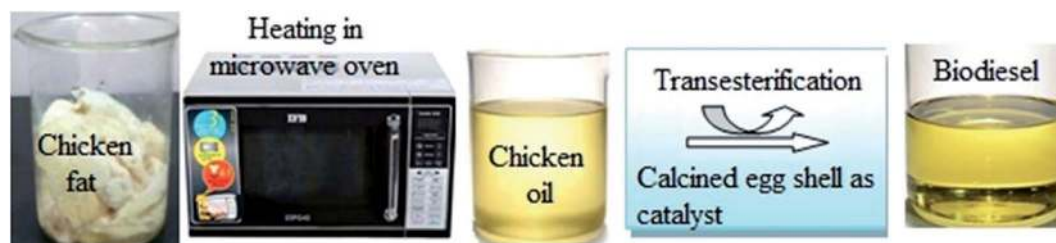
Fig. 14 Microwave-assisted synthesis of FAME using an eggshell catalyst. Reproduced from ref. 190.
