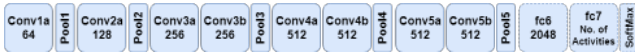
Figure 4. Modified C3D model for vision sensing module. The network parameters in solid line boxes are fixed and those in dashed line boxes are trained.
