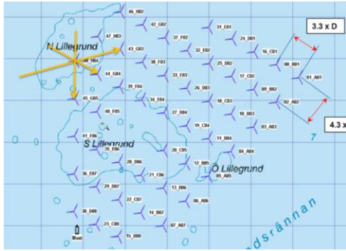
Figure 8. Theoretical wind incoming directions which cause the largest power drop of WTG43-45
