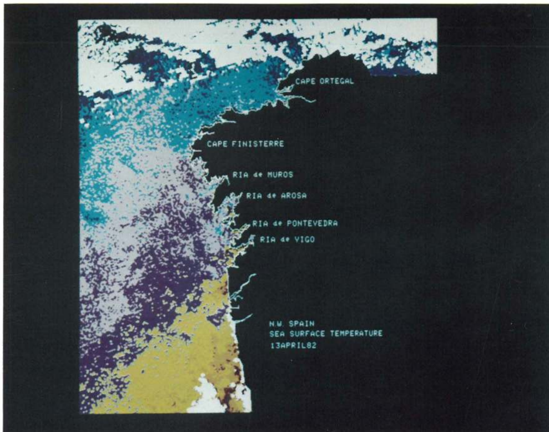
Plate 1. AVHRR sea surface temperature image on April 13, 1982. All satellite images have been remapped to a common transverse Mercator projection having boundaries of 41.0°-44.0°N and 7.5°-10.5°W and are registered to the coastline. Table 1 provides the color code.
