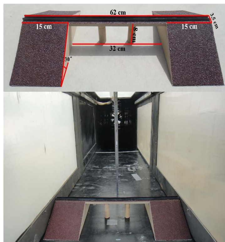
Figure 3. Railway bridge model used in the wind tunnel experiment.
