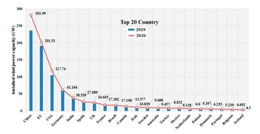
Figure 2. Cumulative installed capacity (CIC) of wind power (MW) 2020 [7,11].
