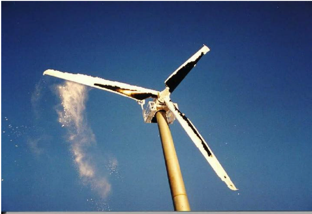
Photograph 8: accumulated ice shedding from black blades
