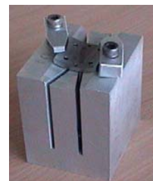
Fig. 8: Welding Fixture for Tail panel with Tail base
