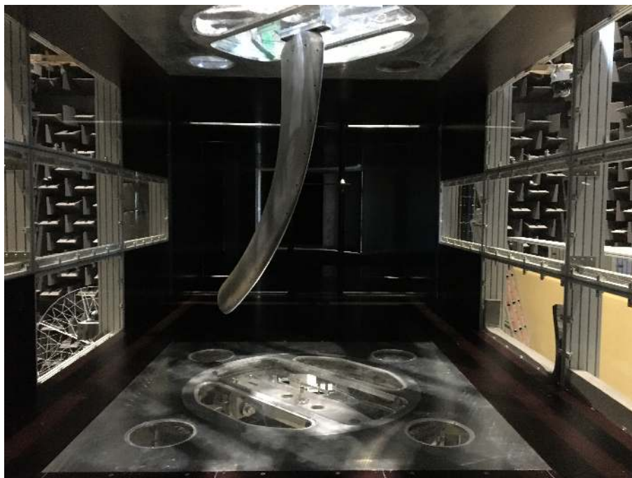
Figure 5. The tip model mounted in the test section of the Poul la Cour wind tunnel.
