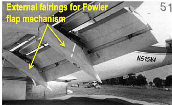
(a) An example of external fairings for Fowler flap mechanism. 7
