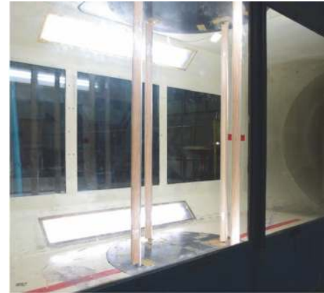
(a) Iced 4-bundled conductors
