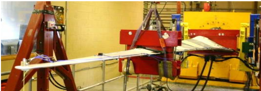
Figure 1. CX-100 blade mounted on test stand.
