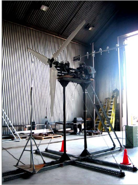
Figure 6-27 Baseline wind turbine blades mounted in the University of Waterloo wind turbine testing facility [89].
