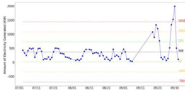
FIGURE 5. The control chart of amount of wind energy generated by No. CK20 (July to September in 2015).
