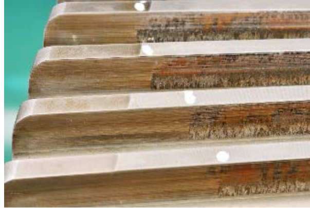
Figure 2.9. Test gearbox high speed stage gear damage. NREL/PIX #19599.
