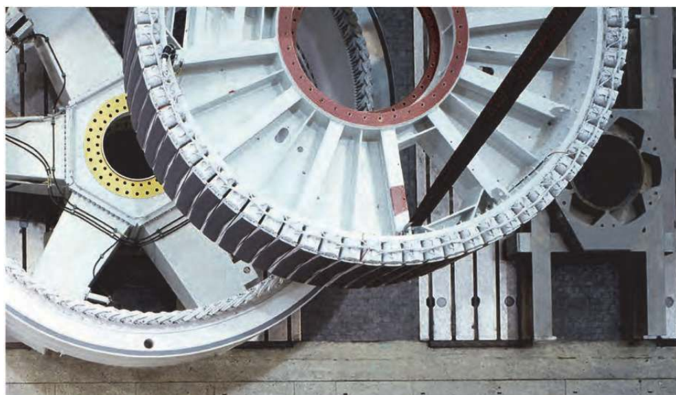
Fig. 5. Rotor and stator of Enercon E-70 wind turbine (Photo: Enercon).
