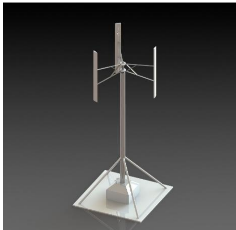
Figure 3. Vertically Axis Hybrid Wind Turbine Construction
