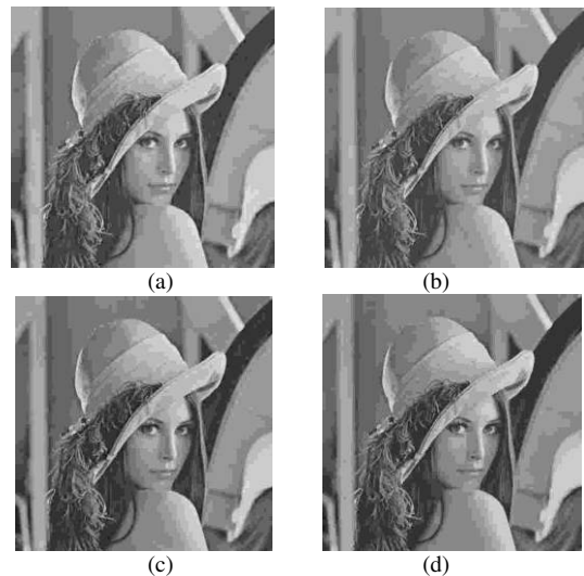
Fig. 11. Lena obtained at 0.20bpp: (a) DCT-JPEG version, with PSNR=29.23dB, (b) APBT-JPEG version, with PSNR=29.44dB, (c) WAPBT1-JPEG version, with PSNR=29.53dB, and (d) WAPBT2-JPEG version, with PSNR=29.43dB.
