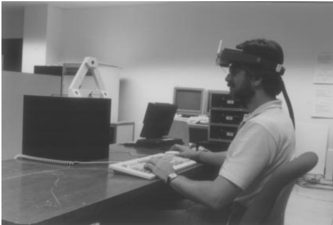
Figure 1: User of our window system wearing a see-through head-mounted display. The large black cube and white triangle are the transmitters for two 3D tracking systems. Tracker receivers are worn on the head-mounted display, waist, and wrist.
