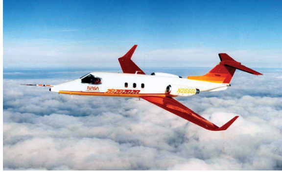
Figure 1.4: The Learjet Longhorn 55 was the first production turbojet powered aircraft to be certified with winglets. [6]
