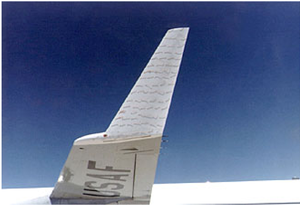
Figure 1.1: In 1979, NASA attached a winglet to a KC135 to evaluate its performance as part of their early winglet research efforts. [21]
