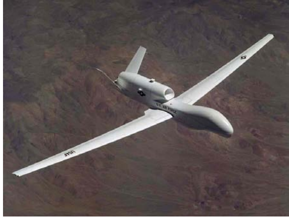
Figure 1.7: The Global Hawk HALE (high altitude long endurance) UAV is built by Northrop Grumman and is used the by US Air Force. It has a wingspan of 130 feet and can carry a payload of 3,000 lbs. It is the largest production UAV currently in service.[27]
