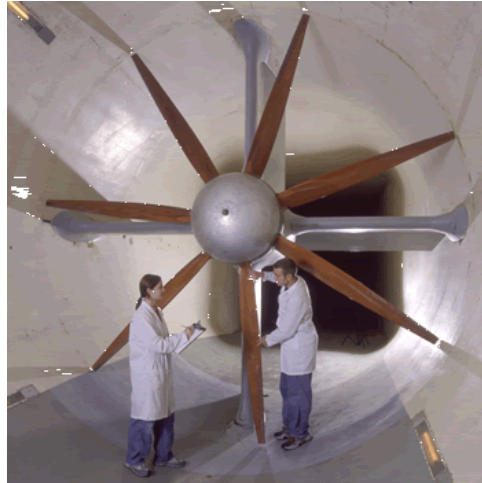
Figure 2.27: The Kistrten Wind Tunnel features 2 massive propellers measuring 11 ft. 4 in. in diameter, with seven blades.[28]
