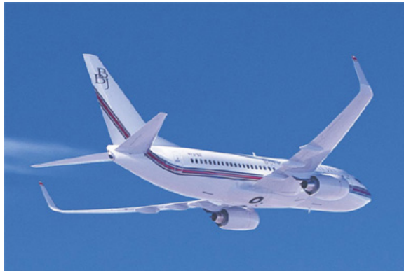
Figure 1.5: The Boeing BBJ (based on the Boeing 737) has blended winglets for improved performance and “aesthetic appeal”. [5]
