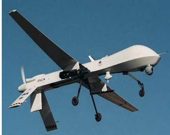
Figure 1.8: The Predator UAV is manufactured by General Atomics. The Predator has a wingspan of 55 feet and can carry both internal and external payloads totaling more than 700 lbs. Nearly 200 Predators are in service.[27]
