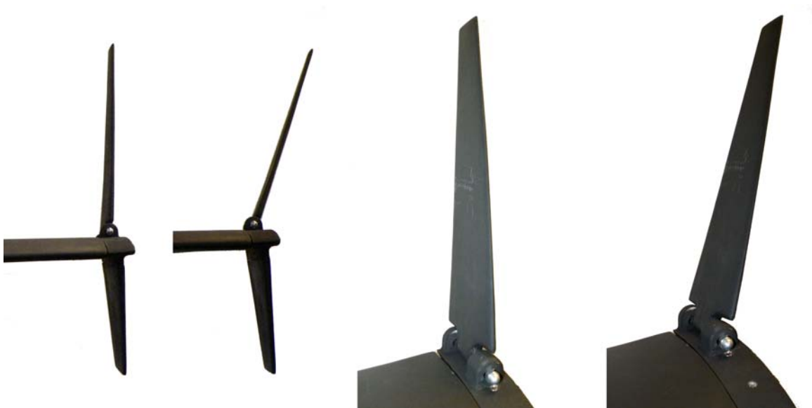
Figure 3.22: Wind tunnel model with a winglet that can be set to variable angles for the cant.
