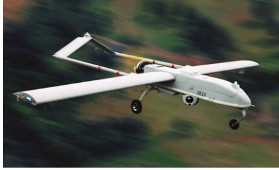
Figure 1.10: The Shadow UAV is manufactured by the AAI Corporation. The Shadow 200 has a wingspan of 20.4 feet, and like the ScanEagle, is launched using a catapult system.[30]
