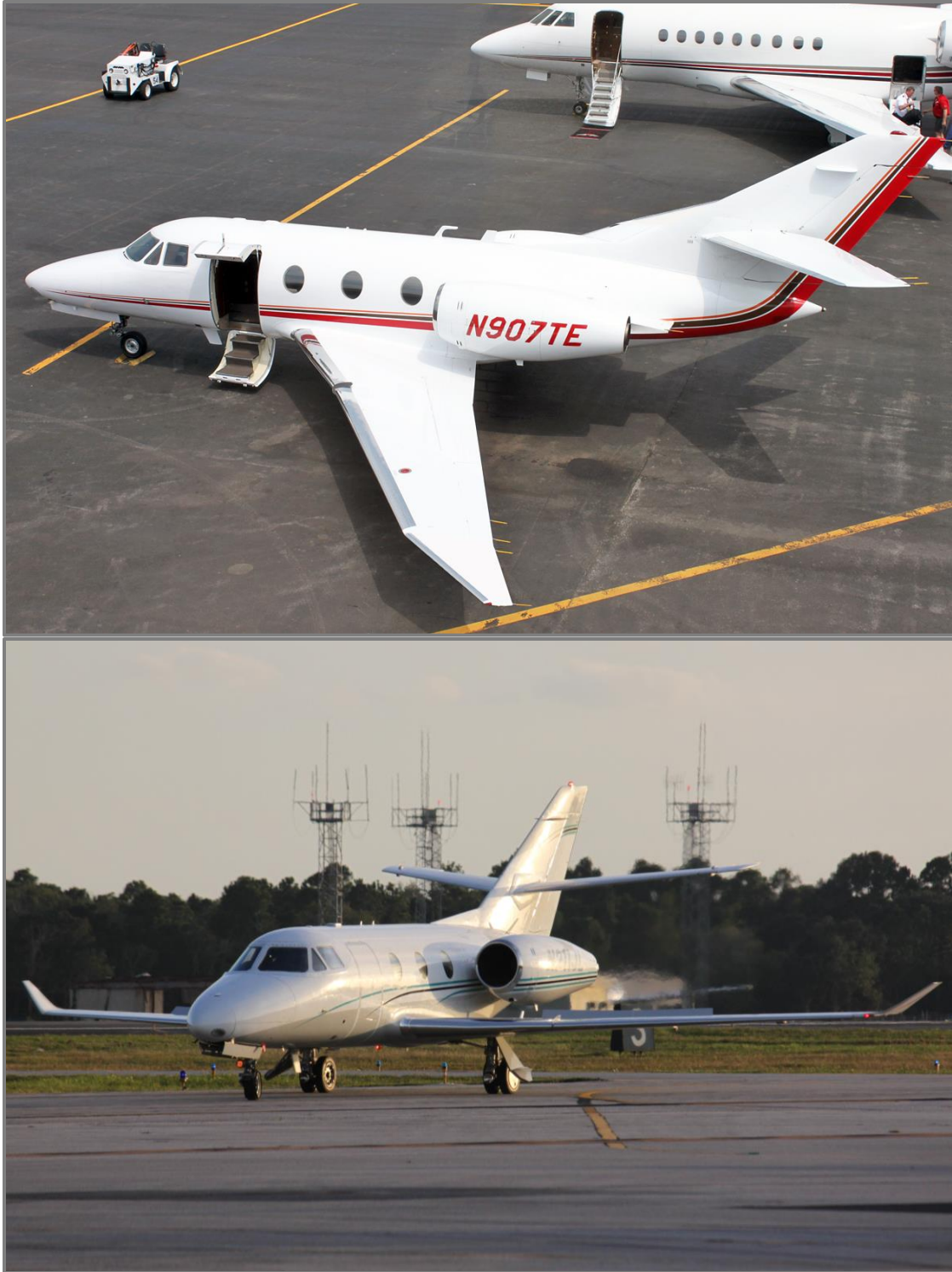
Figure 5.1. Dassault Falcon 10RX and 10LX. This edit shows how the Falcon 10 could appear if a) the recommended raked wingtips b) reduced cant raked winglets would be installed (Pictures by author).
