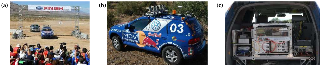
Figure 1: (a) The robot shown at approximately 1:40pm on Oct 8, 2005, as it successfully completes the 132-miles course. (b) View of the car and the roof rack with sensors. (c) The computing system in the vehicle's trunk.
