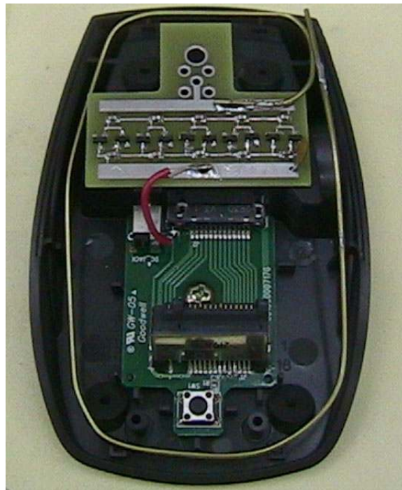
Figure 7.2: Board 2 with Monopole Antenna
