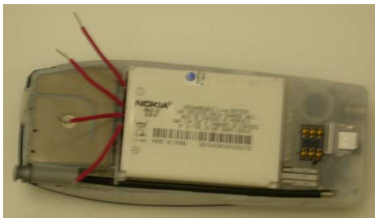
Figure 6.10: Battery In Nokia Phone with External Leads
