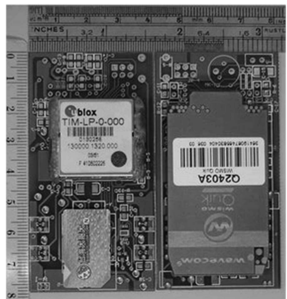
Fig. 7. Top layer (left) and bottom layer (right) of locator's PCS.
