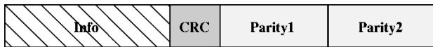
Fig. 1. Arrangement of data in a turbo-coded packet. Unlike RCPC/CRC-coded streams, info bits can be directly decoded if they are not corrupted.
