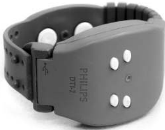
Figure 2 Novel wireless multi sensor bracelet DTI-2
