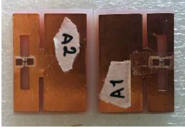
Figure 11. Manufactured prototypes: antennas without support
