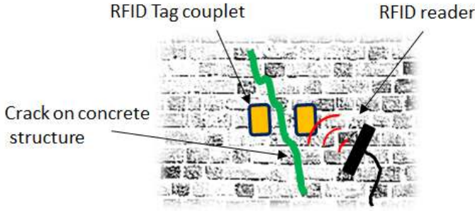
Figure 1. Envisaged system layout: an RFID reader wirelessly interrogates a couplet of RFID tags placed on a cracked wall-like structure and retrieves deformation data
