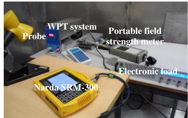
Fig. 5. WPT system: experimental setup.
