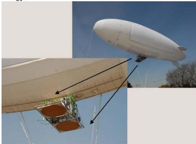
Figure 6 Microwave power transmission experiment with two phase-controlled magnetrons by Kyoto University, whose microwave power was transmitted from the airship in 2009.
