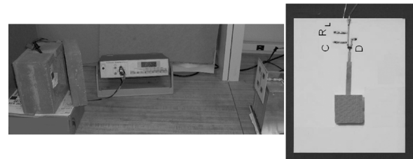
Fig. 5. Photograph of the rectenna measurement setup and the rectenna.
