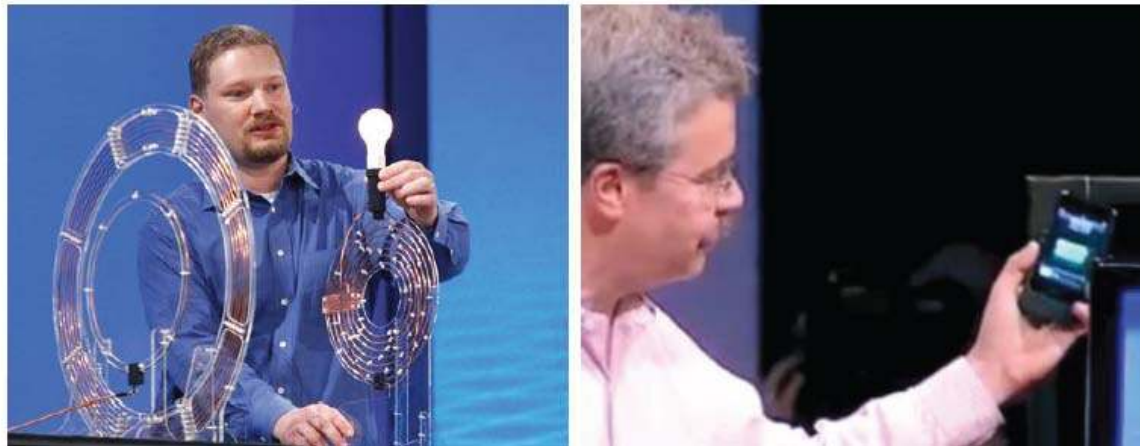
Demonstration of magnetic coupling to power light bulb (Intel Corp.) and charge mobile phones (Witricity Corp.)
