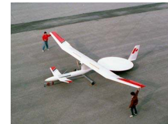
The SHARP unmanned plane receives energy beamed from the ground
