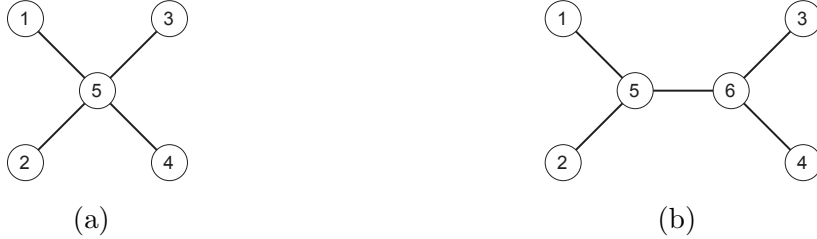
Figure 14: Scenarios when the AHLoS system [63] can use atomic multilateration (a) and collaborative multilateration (b).
