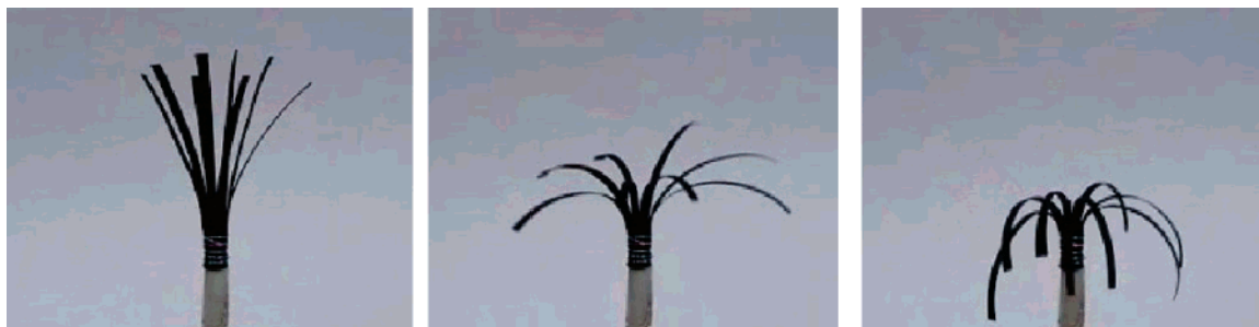
Figure 3. Strips of polypyrrole actuators are arranged in a flower structure. The actuators are shown to bend significantly, their bending direction depending on the voltage polarity ( \pm 1 V). The large displacement that can be obtained using low mass, low power, and low voltage polymer actuators makes them attractive in the development of biologically inspired robots. Photos courtesy of Y. Wu, Intelligent Polymer Research Institute, University of Wollongong.
