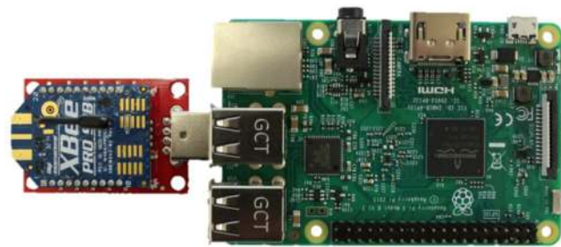
Figure 8. Raspberry Pi with attached XBee coordinator.
