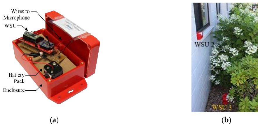
Figure 11. (a) Packaging of WSU for field deployment; (b) Field deployment of WSUs.
