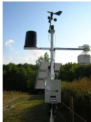
(b) VineSense GPRS Gateway with Weather Sensors
