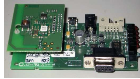
FIGURE 6: Z-Wave node with interface module.
