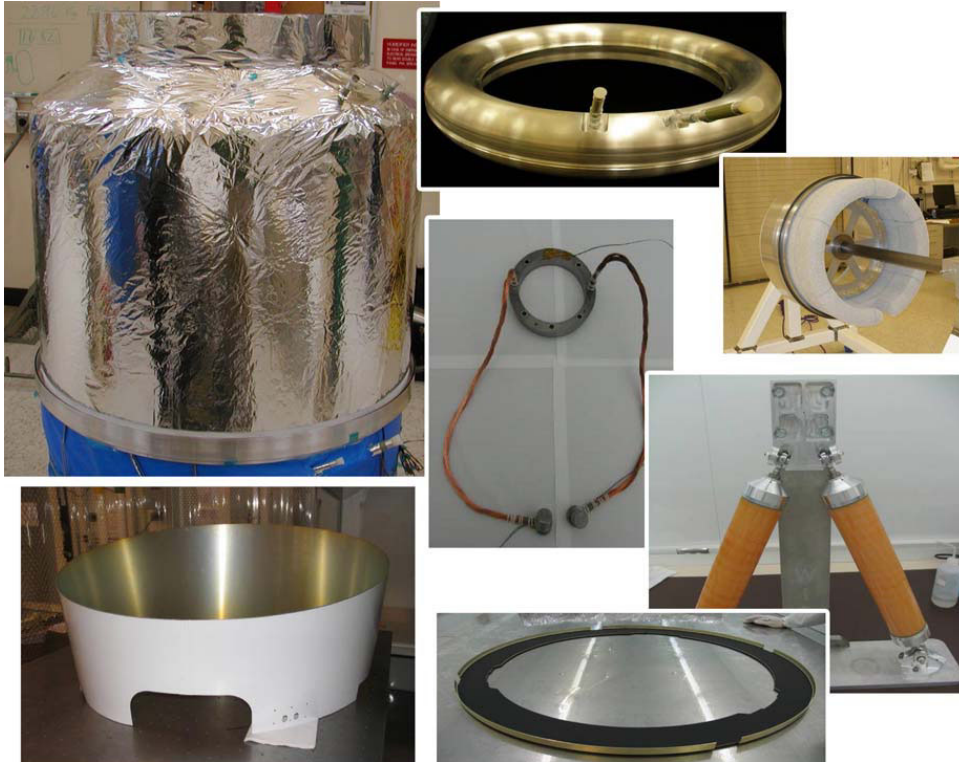
Figure 5. Cryogenic support system hardware. (Clockwise from top left: primary and secondary tank assembly layered with MLI to inner VCS, assembled primary tank, secondary tank heat exchanger installed to the telescope interface flange, bipod assembly, aperture shade radiator, outer aperture shade, primary thermal link.)
