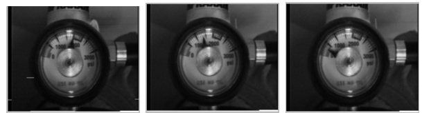
Fig. 12. A mechanical pressure gauge as captured by the WISPCam using the setup in Figure 11. These images could be post-processed to extract the gauge reading, or displayed directly to a human operator.
