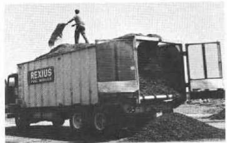
Figure 10. Hogged bark fuel being discharged from a self-unloading truck.
