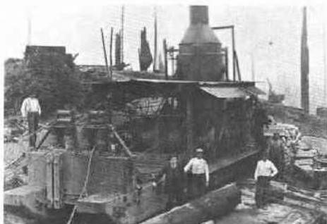
Figure 6. Wood fuel supplied the energy for yarding logs with early steam logging "donkeys".
