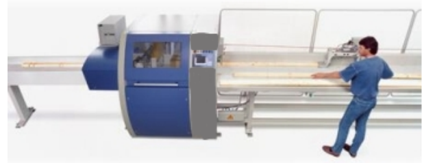
Fig. 1. Example of a cutting optimization machine. The human operator feeds the machine.
